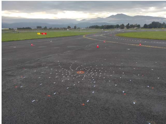
247 microphone multi-arm spiral array
