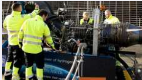
End 2022 RR demonstrated the first engine running on 100% hydrogen (RR @Twitter and BBC)
