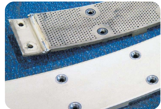
Acoustic Panels: old (top) and new
