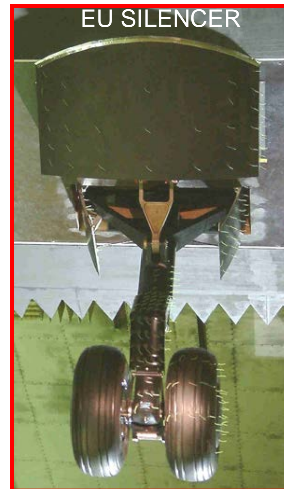
low noise NLG ~ 6.3 dB reduction
