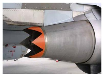
DLH/DLR 2001 – chevron nozzle tested on CFM56-5A-engine:
