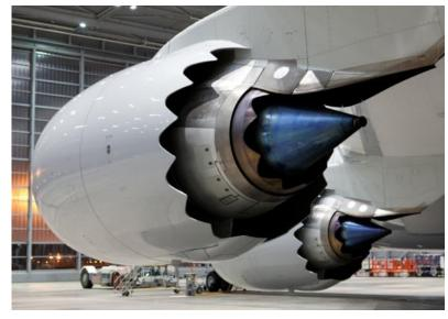
Boeing 747-8I: new GEnx-2B67 engines are equipped with two chevron nozzles: hot stream and cold stream which contribute to significant noise reduction at departure.
