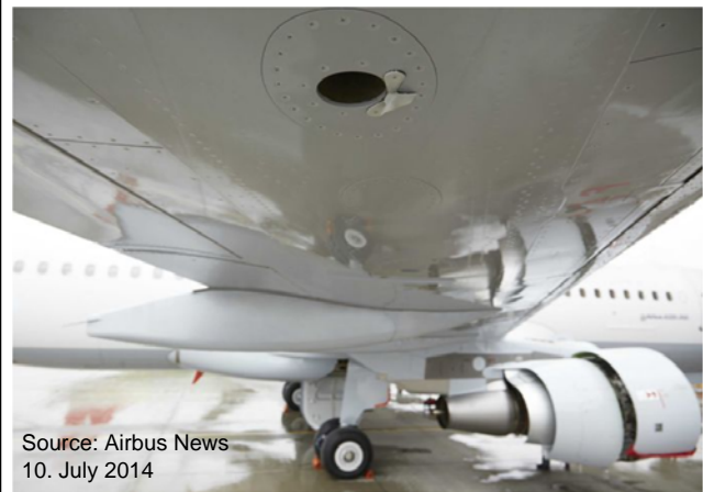
An even quieter approach: Airbus introduces air flow deflectors on the A320 Family
